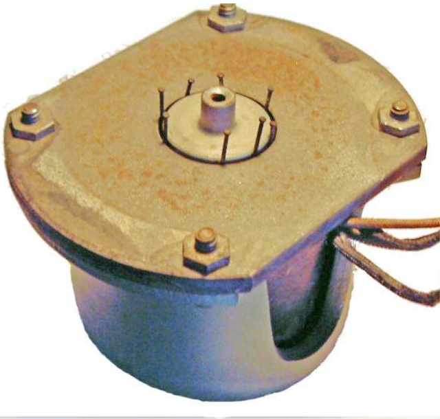
Speaker assembly, with pole clearance wire brads
