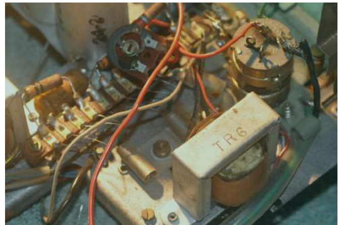
The Kriesler 41-20's output stage
