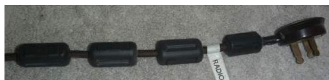
Photo 4. Typical example of an RFI filter on a valve receiver power lead
