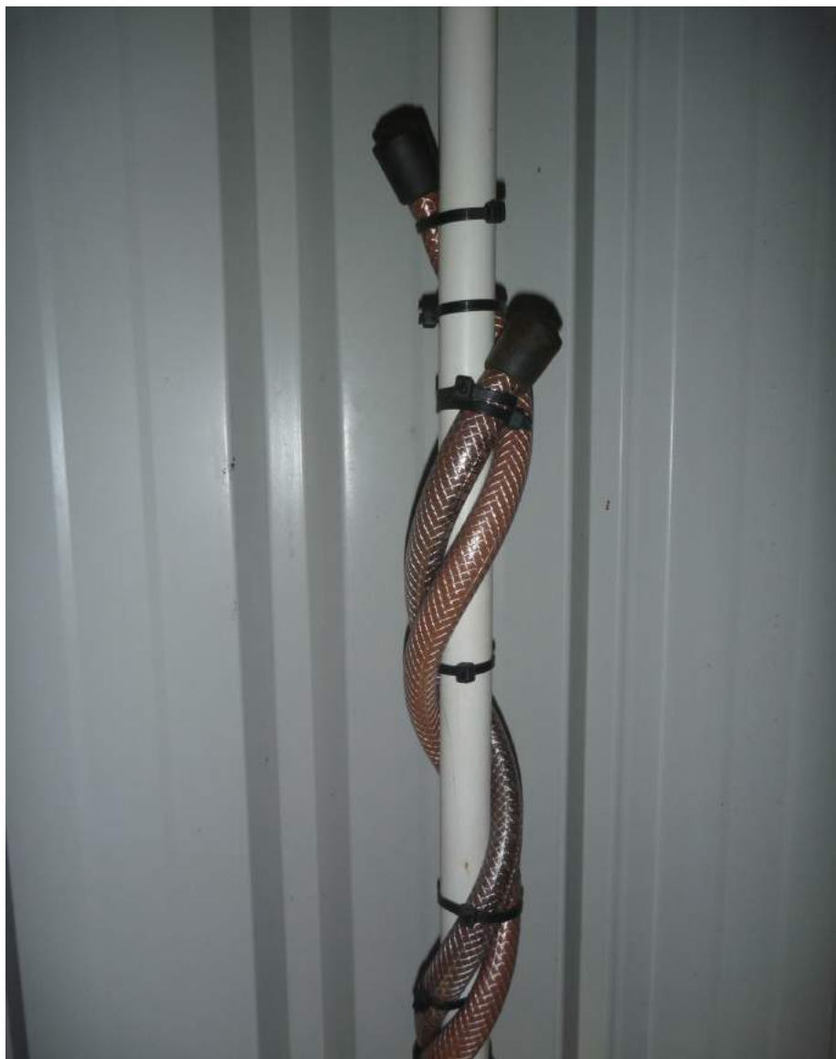
Photo 5. Home made ferric oxide RFI filter
